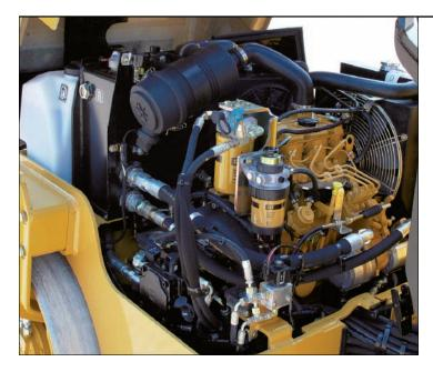
**Power.** The liquid cooled, three cylinder C1.5 engine provides a gross power of 24.4 kW (33.2 hp) for good performance and reliability in all working conditions.
