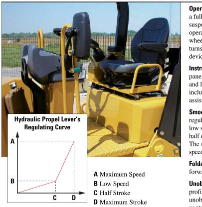
**Operator's Station.** The operator's station incorporates a fully-equipped console and an adjustable sliding suspension seat. Arm and wrist rests provide better operator comfort for day-long productivity. The steering wheel includes a steering knob for easy maneuverability in turns. A 12-volt outlet for plugging in personal electronic devices is also included.
