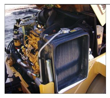
**Easy Access.** The vertical lift engine enclosure allows easy access to the engine oil filter, hydraulic filter, vibe block, radiator and propel pumps, making routine service quicker than ever.
